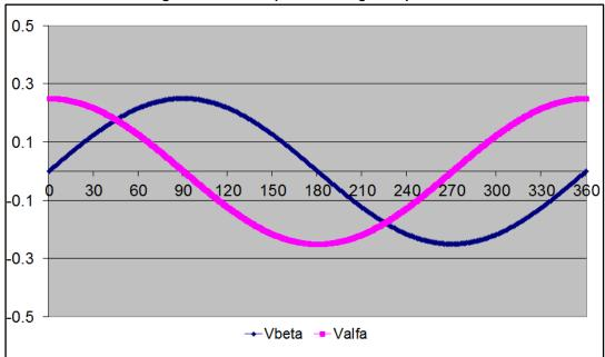
Figure 30:  $V\alpha$  and  $V\beta$  stator voltage components
