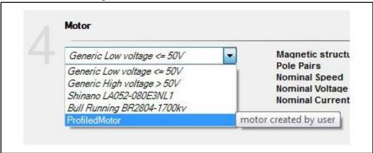
The created project imports the HW settings according to the selected boards and the motor settings according the Motor profiler results; it also imports other settings like PWM frequency and startup acceleration used during the Motor Profiler procedure.
