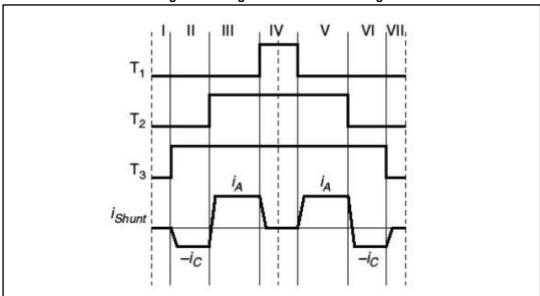
If the stator-voltage demand vector lies in the boundary space between two space vector sectors, two out of the three duty cycles will assume approximately the same value. In this case, the seven subperiods are reduced to five subperiods.
