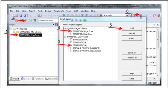
Figure 92: Workspace batch build for Keil uVision
