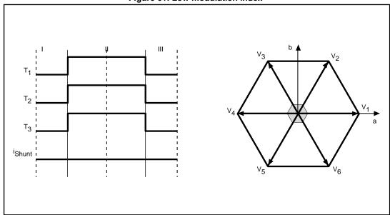
Figure 61: Low modulation index
