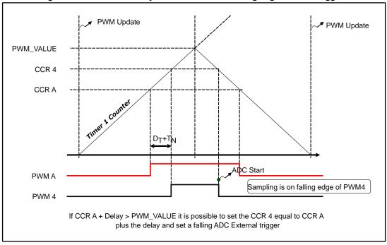
In this way, supposing that the sampling point must be set before the counter overflow, that is, when the TIM1 counter value matches the OCR4 register value during the up counting, the A/D conversion sequence for current sampling are started. If the sampling point must be set after the counter overflow, it's necessary set a falling edge ADC external trigger. Thus, when the TIM1 counter matches the OCR4 register value during the down counting, the A/D sampling are started.
