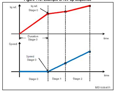
Figure 113: Example of rev-up sequence
