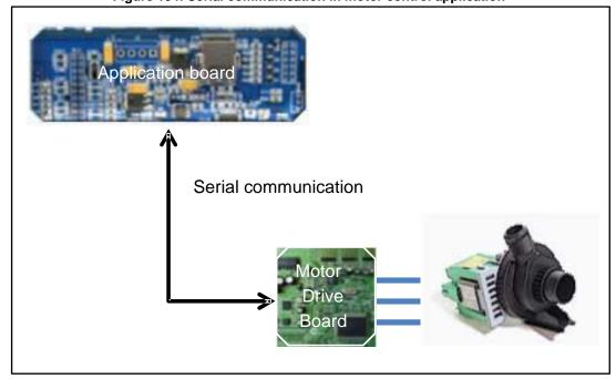
Figure 134: Serial communication in motor control application
