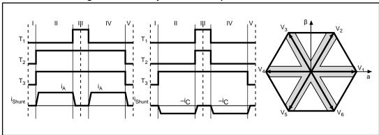
Figure 60: Boundary between two space-vector sectors
