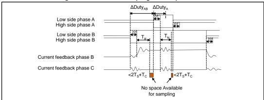
Figure 57: Two current samplings cannot performed
