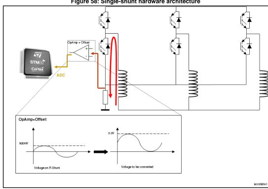
Figure 58: Single-shunt hardware architecture
