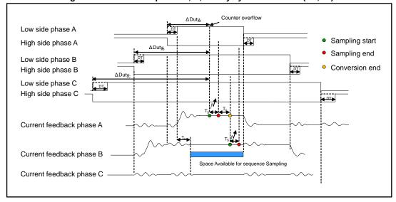
Figure 53: Low side of phase A, B, C duty cycle > DT + max(TN,TR)
