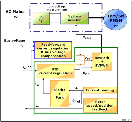
Figure 22: Feed-forward current regulation
