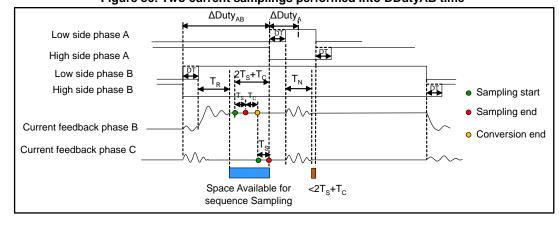
Figure 56: Two current samplings performed into DDutyAB time
