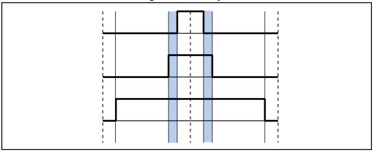
The voltage-demand vector lies in a region called Boundary 2 when two duty cycles differ from each other by less than  $D_{MIN}$ , and the third is smaller than the other two and differs from them by more than  $D_{MIN}$ . This is represented in *Figure 64: "Boundary 2"*.
