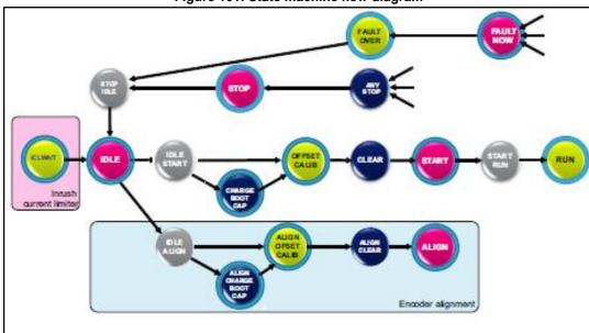
Figure 101: State machine flow diagram
