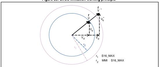
Figure 33: Circle limitation working principle
