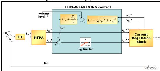
Figure 23: Flux-weakening operation scheme
