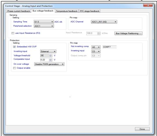
Figure 75: STMCWB windows related to ADC/COMP settings for DC bus Voltage
