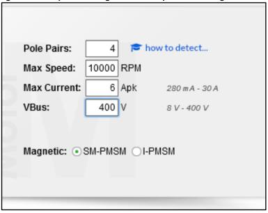
If the motor has an internal permanent magnet, select I-PMSM. You must also input the Ld/Lq ratio.
