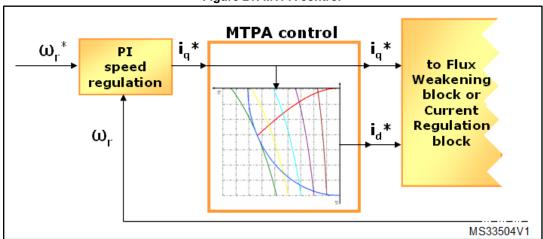
In all cases, by acting on the direct axis current  $i_{ds}$ , the magnetic flux can be weakened so as to extend the achievable speed range. As a consequence of entering this operating region, the MTPA path is left (see Section 6.8: "Flux-weakening control" for details about the flux-weakening strategy).
