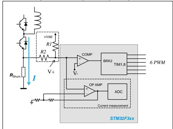
Figure 70: Current sensing network using external gains
