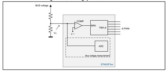
Figure 73: Overvoltage protection network
