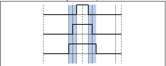
If the voltage-demand vector lies in Boundary 1 or Boundary 2 region, a distortion must be introduced in the related PWM signal phases to sample the motor phase current.
