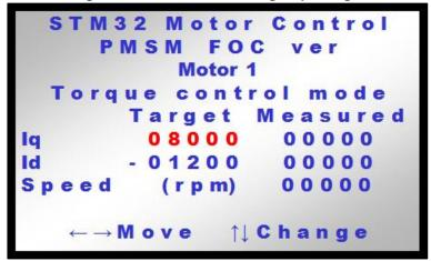
From the previous screen (*Figure 116: "LCD screen for Target Iq settings"*), if the joystick is moved to the right, the Target I<sub>d</sub> current component becomes highlighted (in red). This parameter can now be modified by moving the joystick up/down. Once the motor Start command has been issued, the Target I<sub>d</sub> can be changed in runtime while the measured Id current component is shown in the Measured field.
