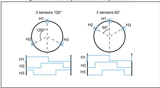
Figure 85: 60° and 120° displaced Hall sensor output waveforms
