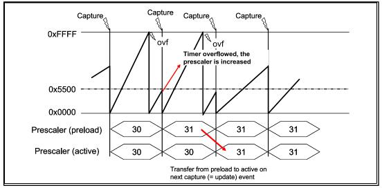
The prescaler modification is done in the capture interrupt, taking advantage of the buffered registers: the new prescaler value is taken into account only on the next capture event, by the hardware, without disturbing the measurement.
