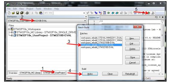
Figure 91: Workspace batch build for IAR EWARM IDE
