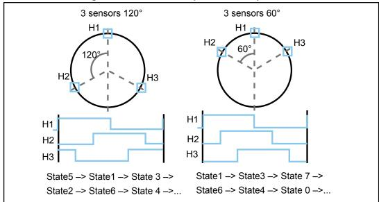
Figure 80: Hall sensors, output-state correspondence
