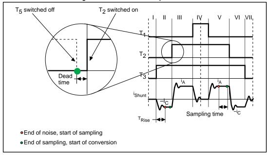
The voltage-demand vector lies in a region called the Regular region when the three duty cycles (calculated by space vector modulation) inside a PWM pattern differ from each other by more than D<sub>MIN</sub>. This is represented in *Figure 62: "Regular region"*.
