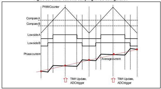
Figure 68: Stator currents sampling in ICS configuration
