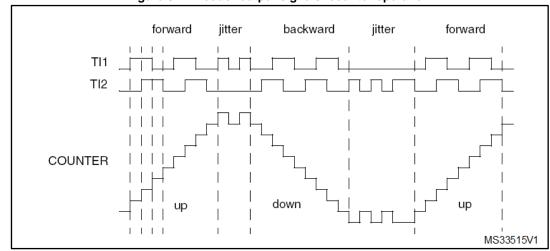
Figure 87: Encoder output signals: counter operation
