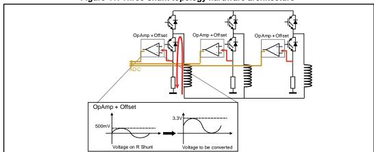
Figure 41: Three-shunt topology hardware architecture
