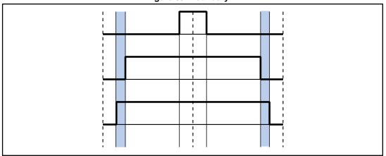
The voltage-demand vector lies in a region called Boundary 3 when the three PWM signals differ from each other by less than  $D_{MIN}$ . This is represented in *Figure 65: "Boundary 3"*.
