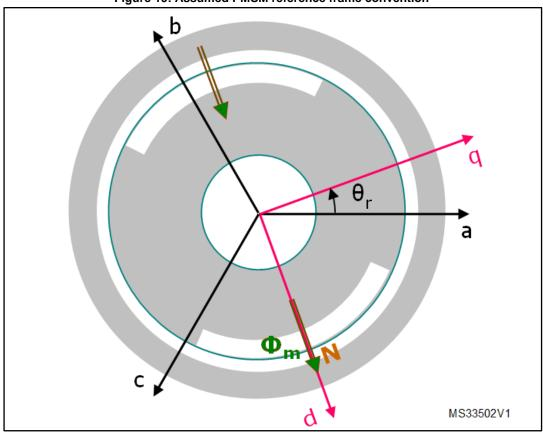
With reference to *Figure 18: "Assumed PMSM reference frame convention"*, the motor voltage and flux linkage equations of a PMSM (SM-PMSM or IPMSM) are generally expressed as:
