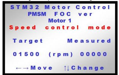
From the menu screen shown in *Figure 118: "Speed control main settings"*, moving the joystick to the right selects the Target speed (parameter highlighted in red). Once selected, the parameter can be incremented/decremented by moving the joystick up/down. The motor can then be started simply by pressing the joystick. When the motor is on, the target speed can still be modified.
