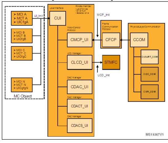
Figure 130: User interface block diagram
