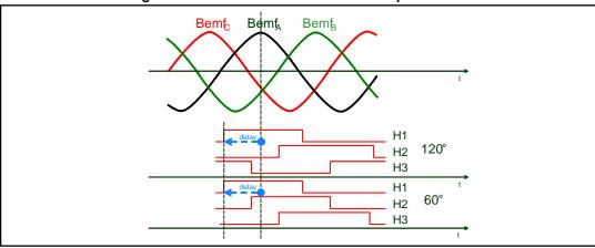
Figure 86: Determination of Hall electrical phase shift
