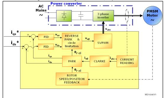
Figure 16: Basic FOC algorithm structure, torque control
