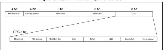
Figure 131: User interface configuration bit field
