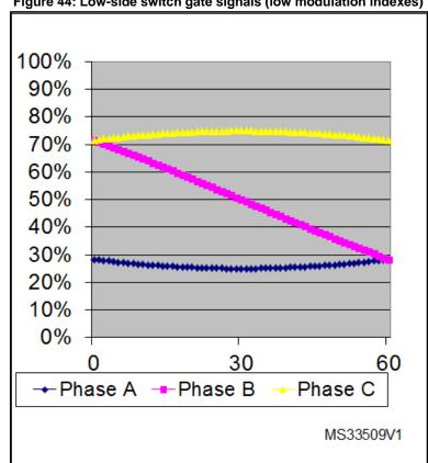
Figure 44: Low-side switch gate signals (low modulation indexes)
