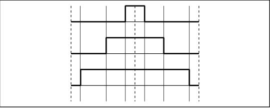
The voltage-demand vector lies in a region called Boundary 1 when two duty cycles differ from each other by less than  $D_{MIN}$ , and the third is greater than the other two and differs from them by more than  $D_{MIN}$ . This is represented in *Figure 63: "Boundary 1"*.
